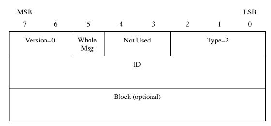
The Resend Request PDU is encoded as follows:
