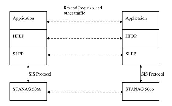
In order for HFBP broadcast to work, both sender and receiver will be connected to two STANAG 5066 stacks. This split will be done by the HFBP layer, so that this is transparent to the broadcast application.
